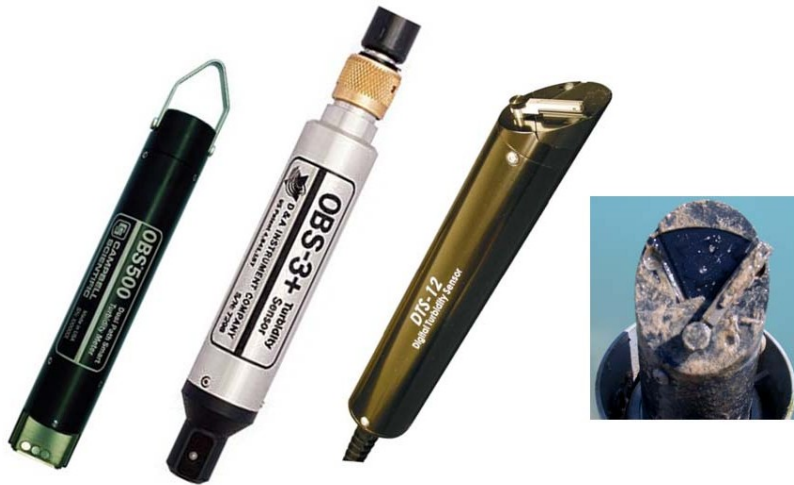
Figure 3-2: Examples of single parameter turbidity instruments (CSC, 2012; FTS, 2012)
