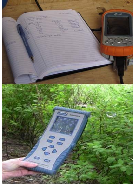
Figure 3-4: Hand held display units for viewing water quality data in-situ
